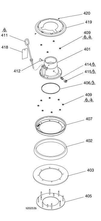
$\triangle$  Apply grease to hold ring (406) in place during assembly.
